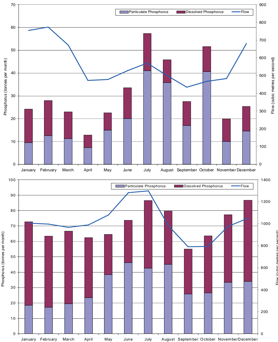
Figure 7.6: Seasonal variation in total phosphorous load from the Saskatchewan River (top figure) (monthly average for non-missing years from 1994 to 2007), and the Winnipeg River at Point du Bois (bottom figure) (monthly average from 1994 to 2007).
