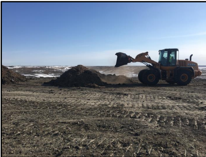
Photograph 2: A front-end loader mixes the feedstocks together at the appropriate ratios (February, 2017).
