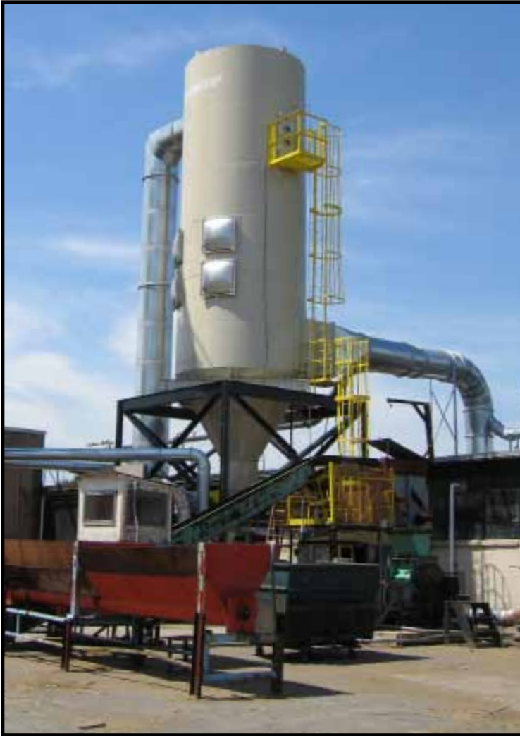
Model 12HVP368 on Wood Dust - Lumber Industry
