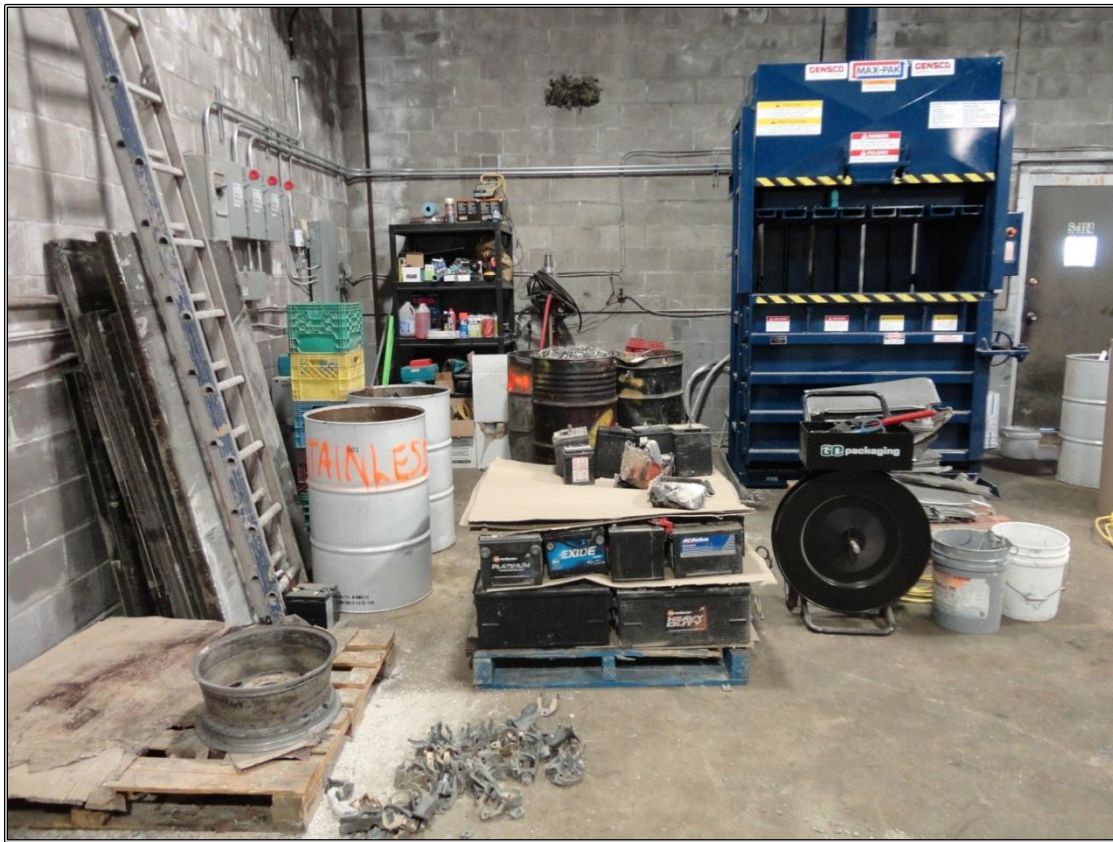
Figure 9: Current indoor waste battery storage area contained within the non-ferrous warehouse. 5 to 7 pallets of waste lead acid batteries are stored for transfer at any given time. Duration of storage ranges from 1 week to 3 months (maximum). The average duration of storage is 2 weeks. A battery acid spill kit will be on hand for any incidents of leakage or spillage. Pallets are loaded to a maximum of 3 levels.
