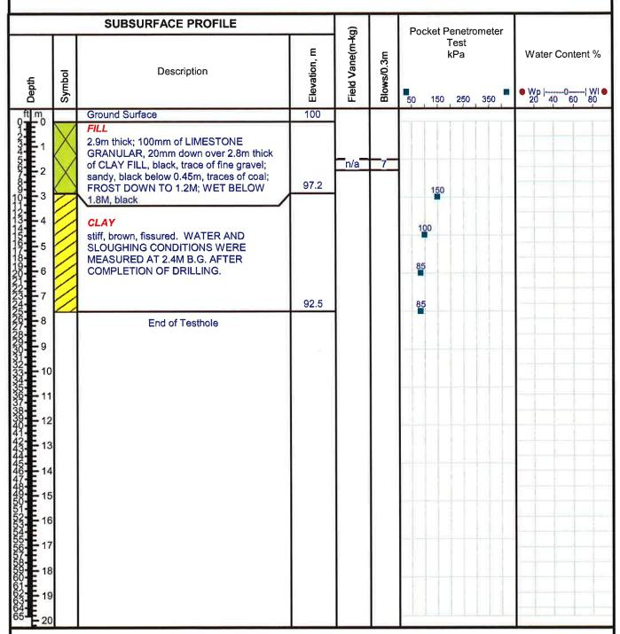
**Drill Method: Continuous Auger**
