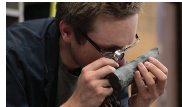
Exploration of the Footwall Deep Project continues underground on the 3600-foot level. Drill core from approximately 6,000 feet below surface is brought to surface for analysis.
