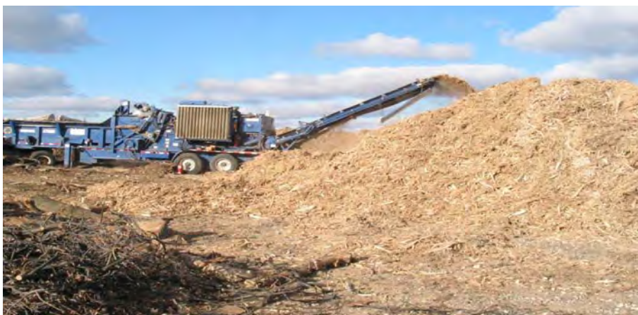
Photo 1-6: Chipping of residue wood from wood wastes for recycling
