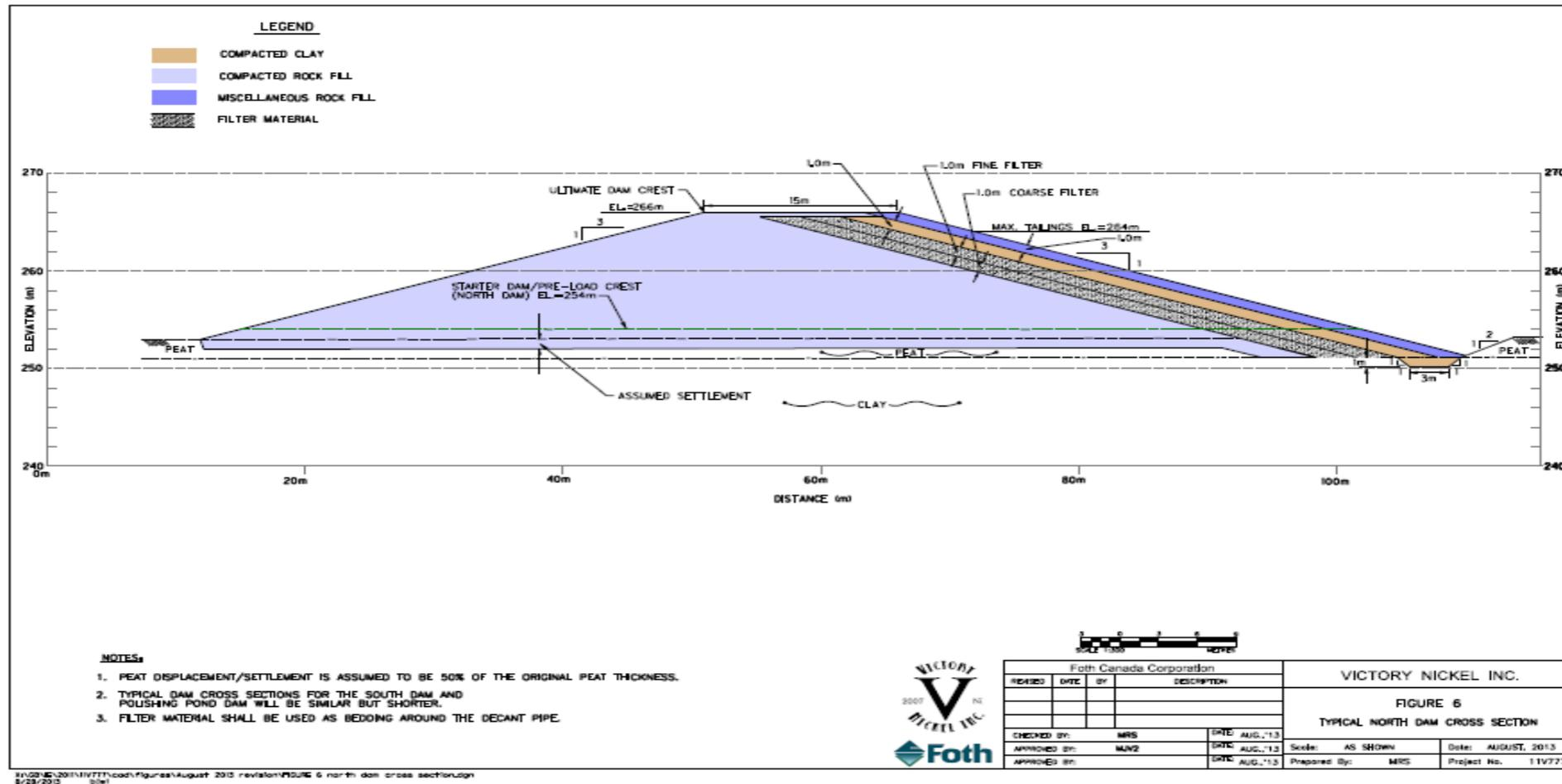
Figure 2.13-6 Typical North Dam Cross Section
