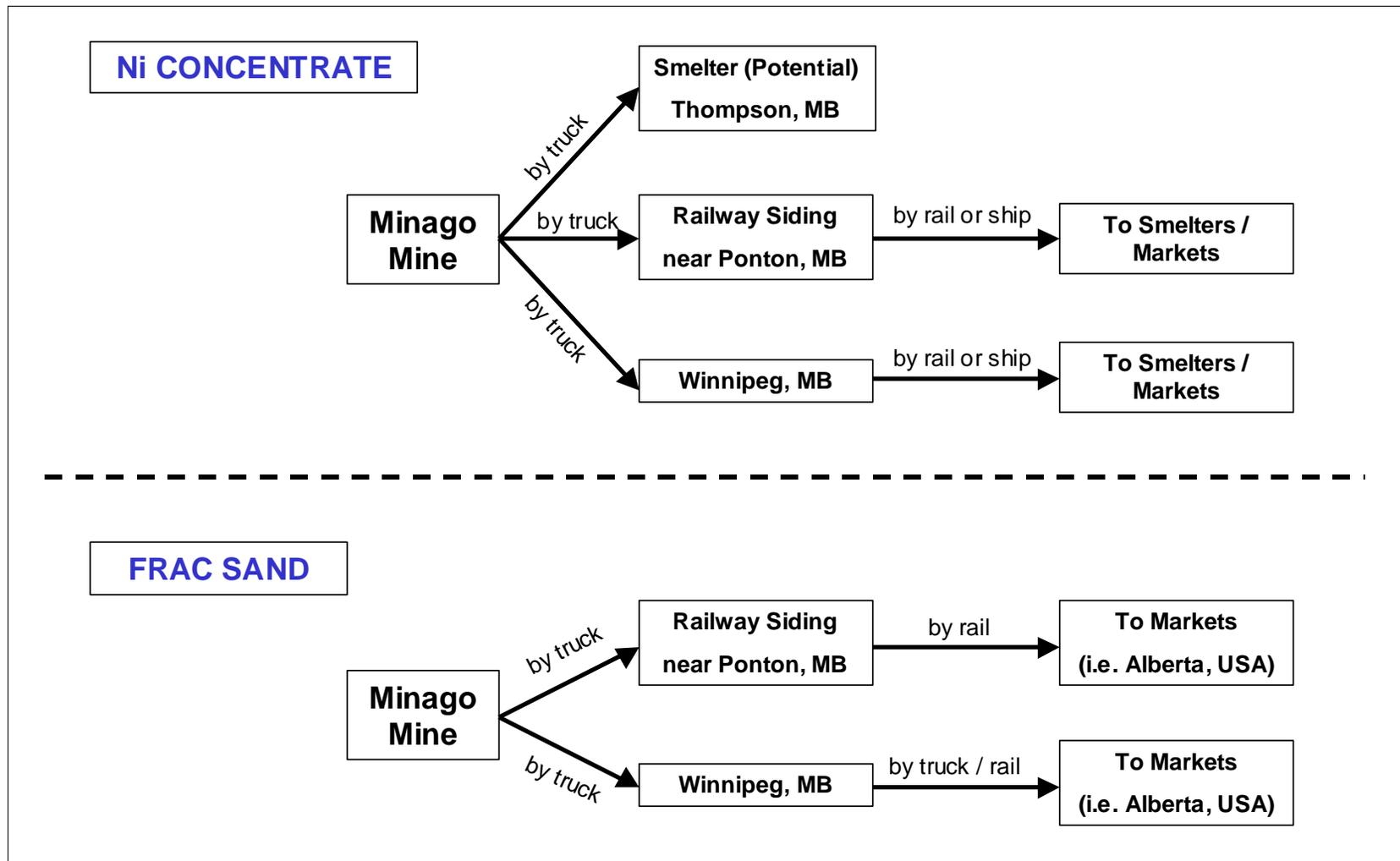
Figure 2.16-2 Concentrate and Frac Sand Haulage Routes
