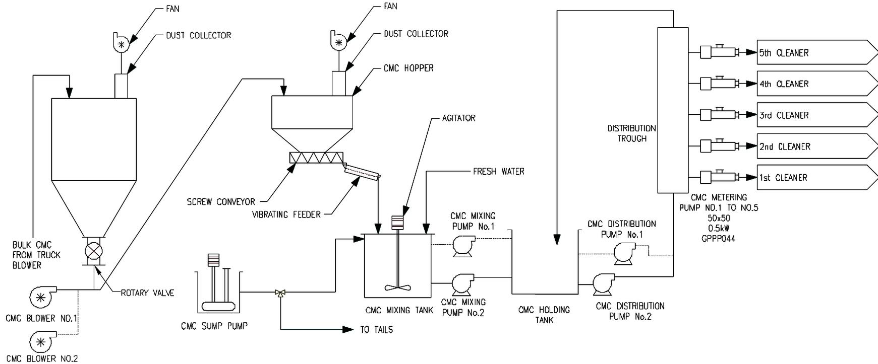
Figure 2.10-2 CMC Reagent Flow Sheet
