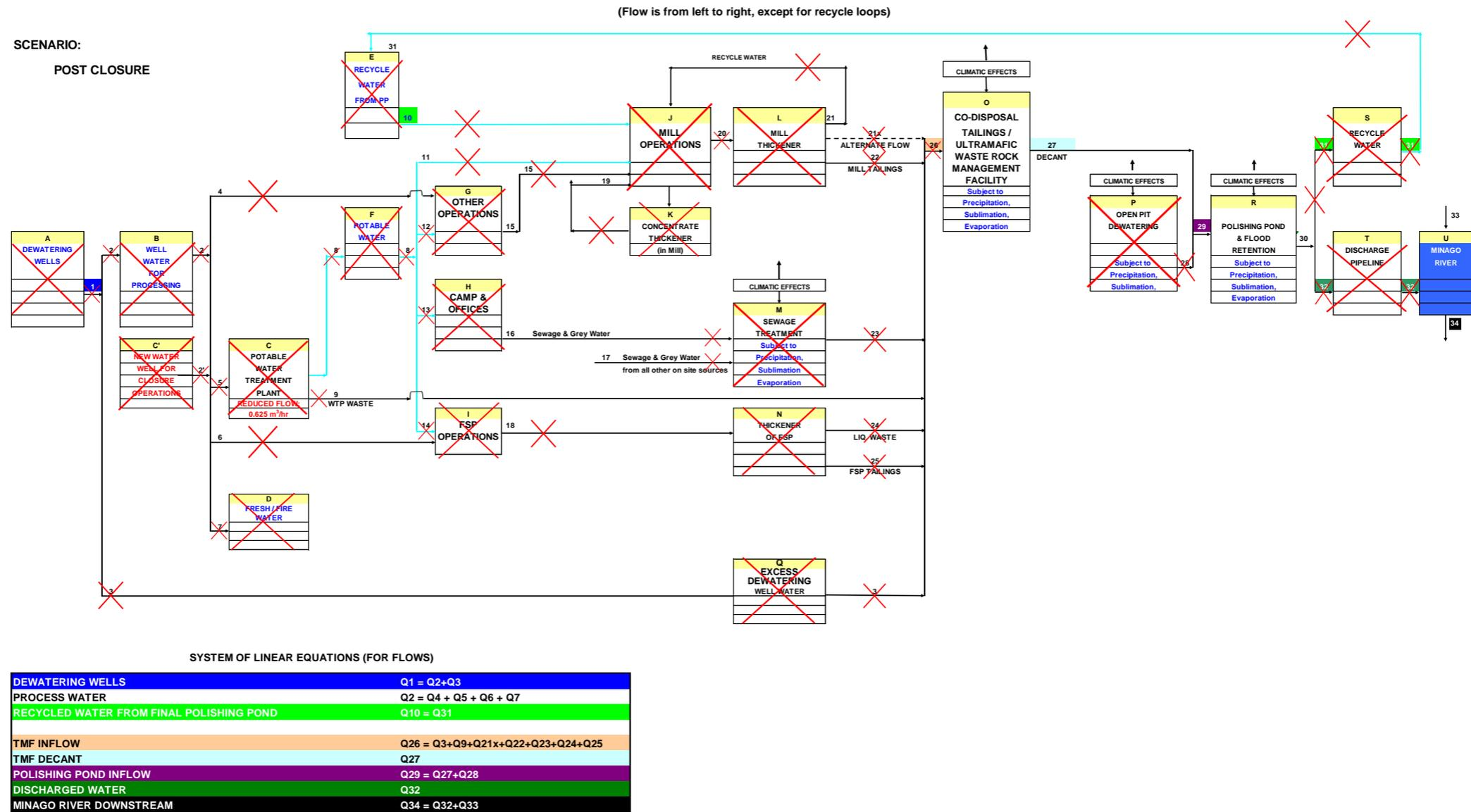
Figure 2.14-5 Post Closure Water Management System
