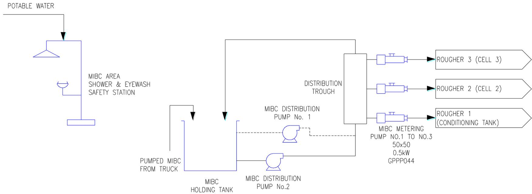
Figure 2.10-5 MIBC Reagent Flow Sheet
