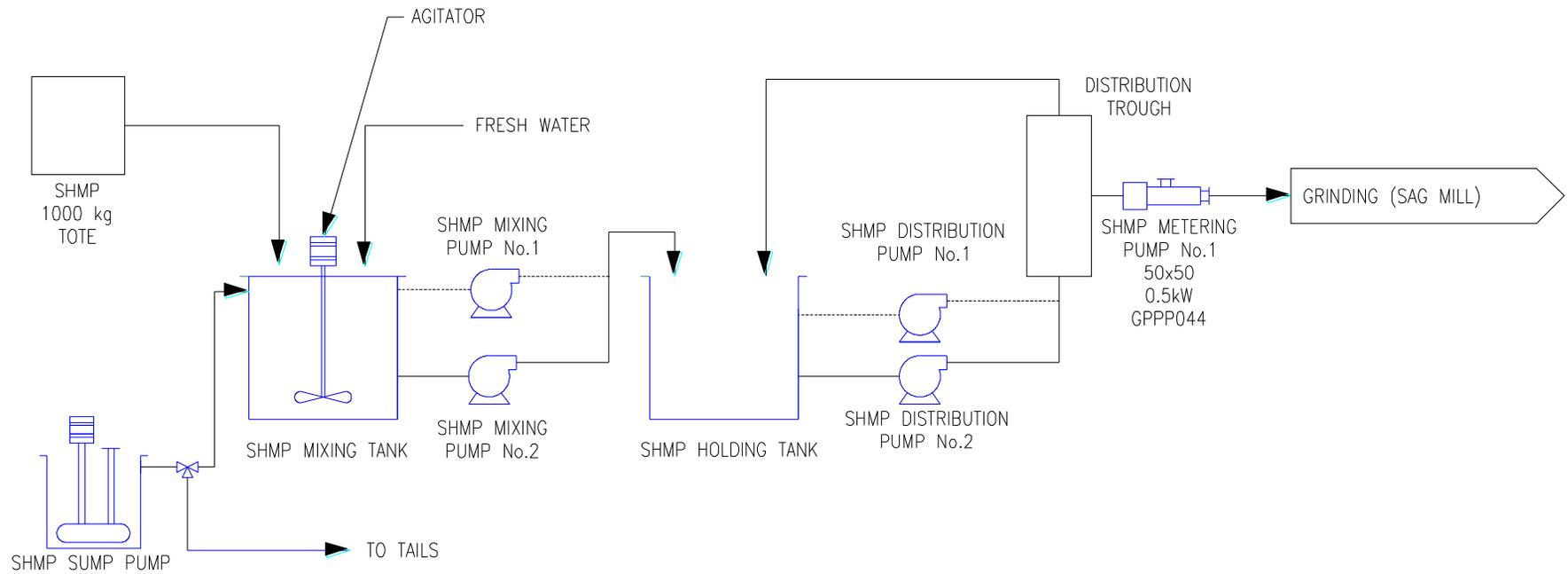
Figure 2.10-4 SHMP Reagent Flow Sheet
