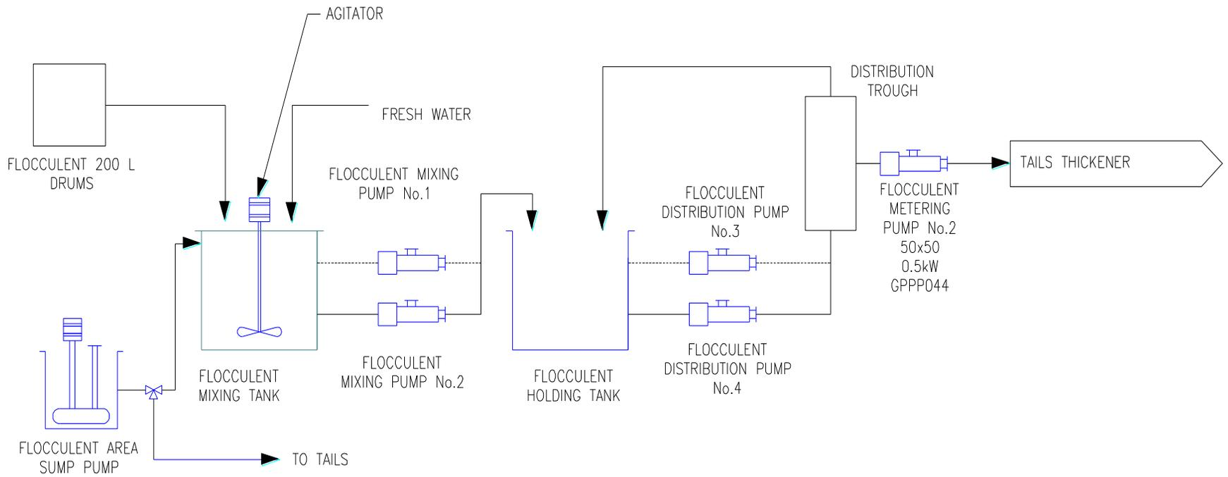
Figure 2.10-7 Tailings Flocculent Flow Sheet
