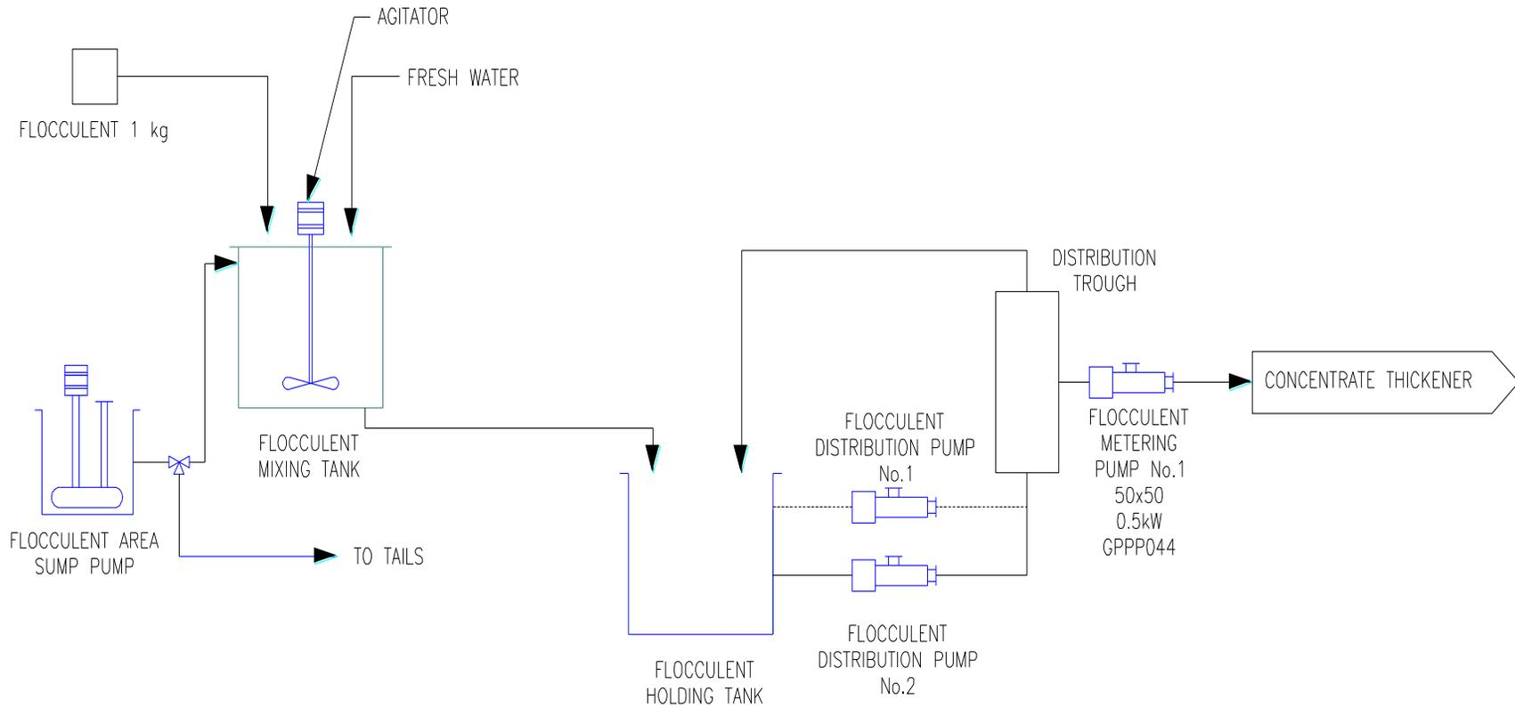
Figure 2.10-6 Concentrate Flocculent Flow Sheet
