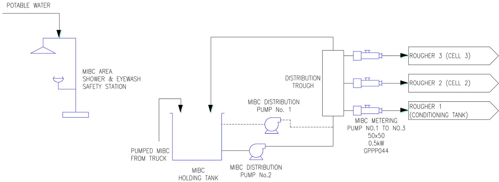
Figure 2.10-5 MIBC Reagent Flow Sheet
