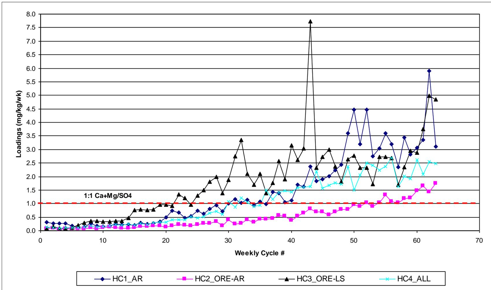
Figure 2.8-11 Ca+Mg/SO<sub>4</sub> Ratios for Minago Phase I Waste Rock Kinetic Tests
