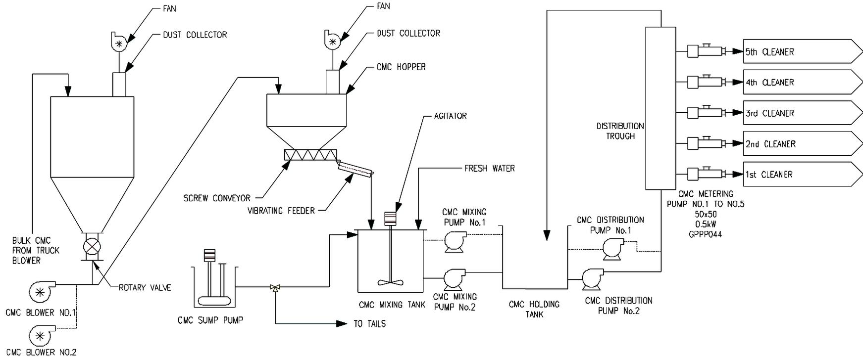
Figure 2.10-2 CMC Reagent Flow Sheet
