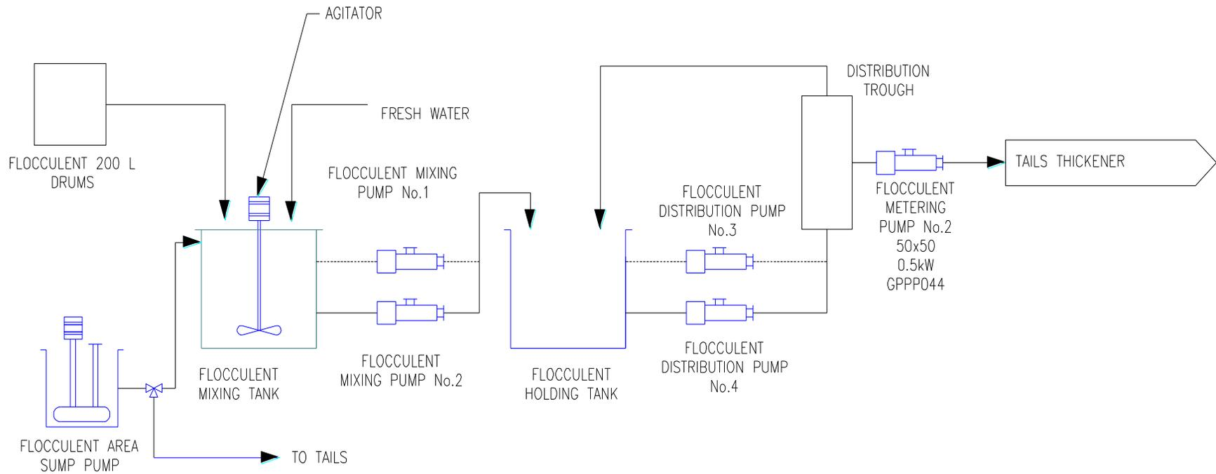
Figure 2.10-7 Tailings Flocculant Flow Sheet
