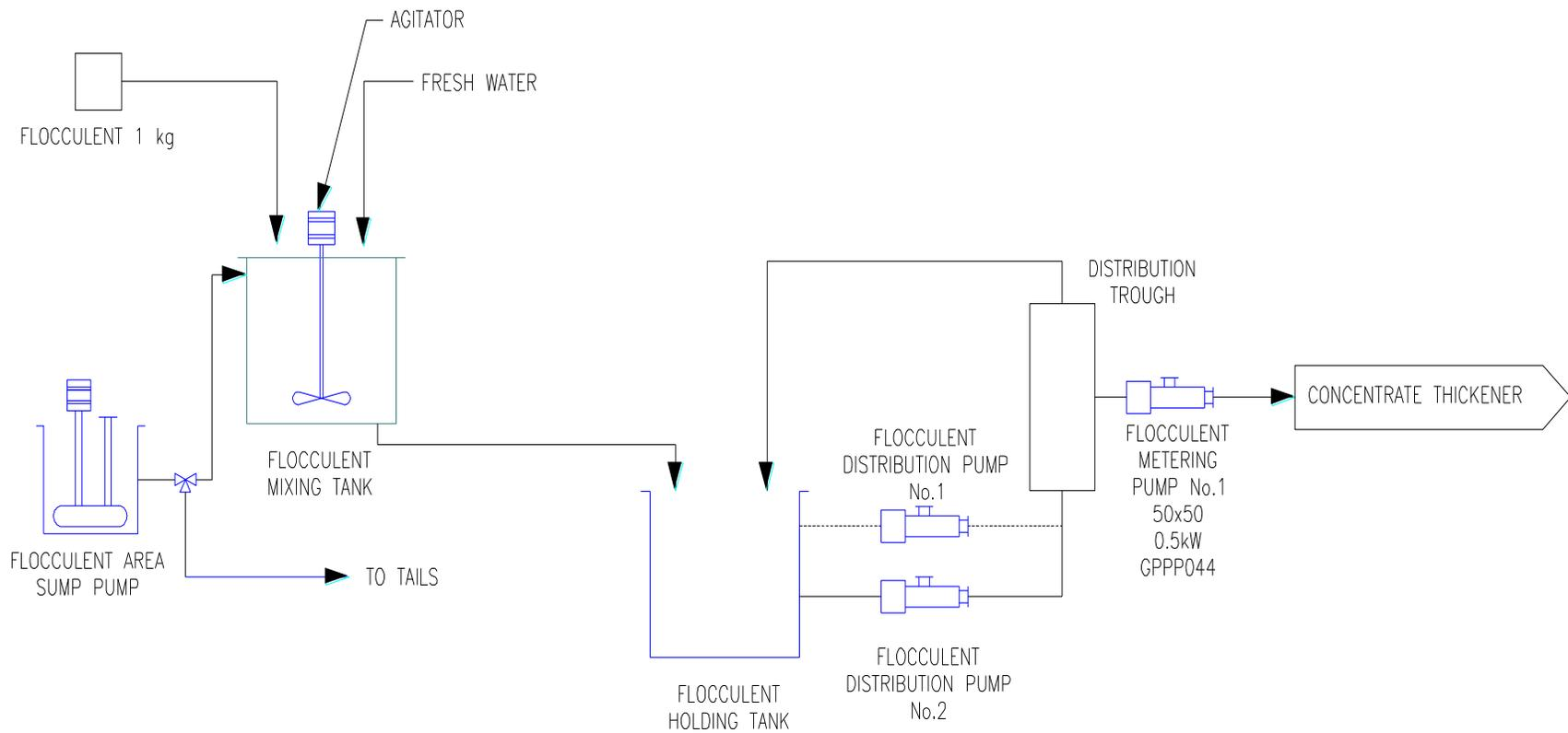
Figure 2.10-6 Concentrate Flocculant Flow Sheet
