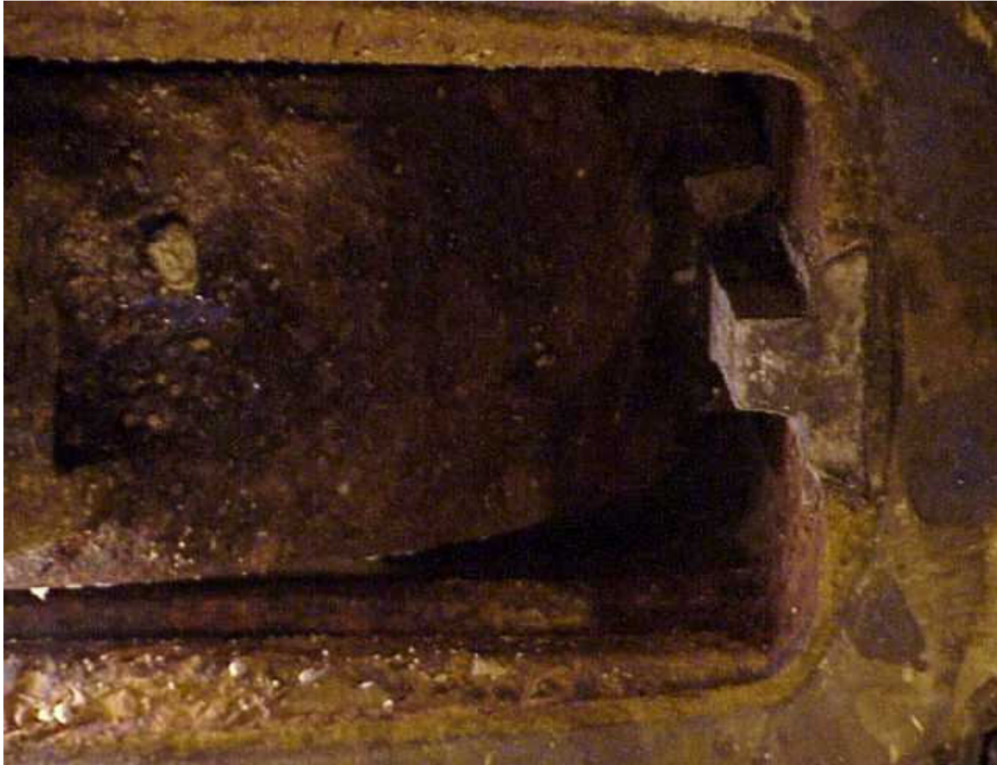
Photo shows valve guide in place on the lower portion of the valve body
