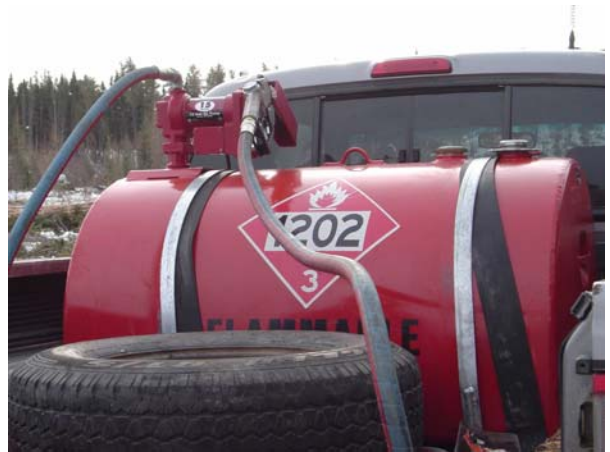
Ensure slip tanks are secured in the truck box and have a cradle to secure the nozzle
