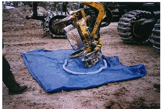
Felling head ready for maintenance without contaminating soil
