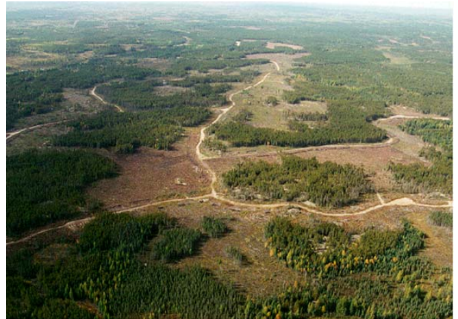
Good locations of roads in this summer block. Road system will be reused 10-15 years later to harvest residual blocks. Note: Layout to meet wildlife guidelines.
