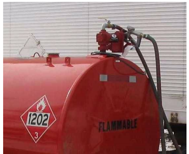
Nozzle is properly secured in the cradle and minimizes the risk of spillage
