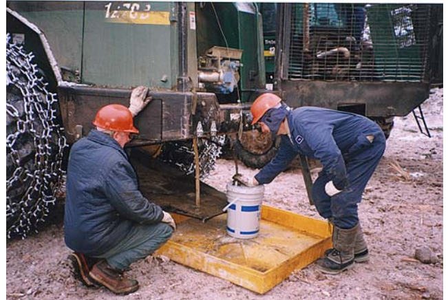
Mechanics using a drain hose to safely drain used oil – note containment tray
