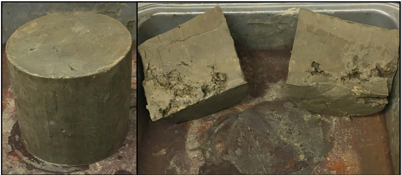
PHOTOGRAPH #4: Sample S5 after hydraulic conductivity testing.
