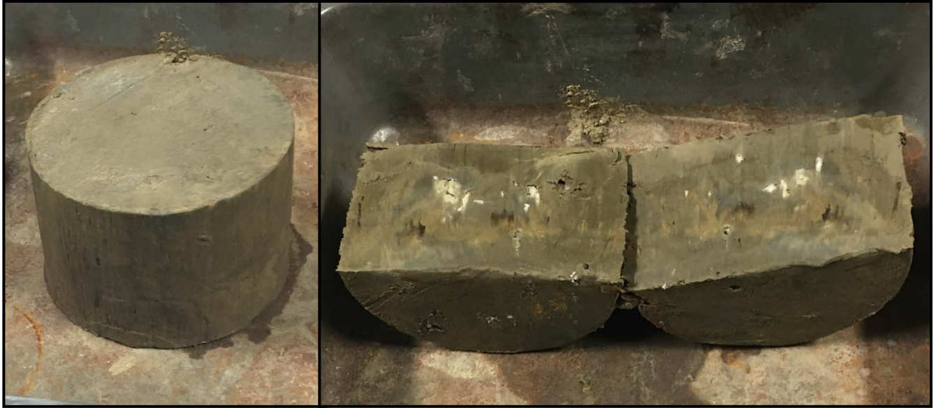
PHOTOGRAPH #5: Sample S6 after hydraulic conductivity testing.
