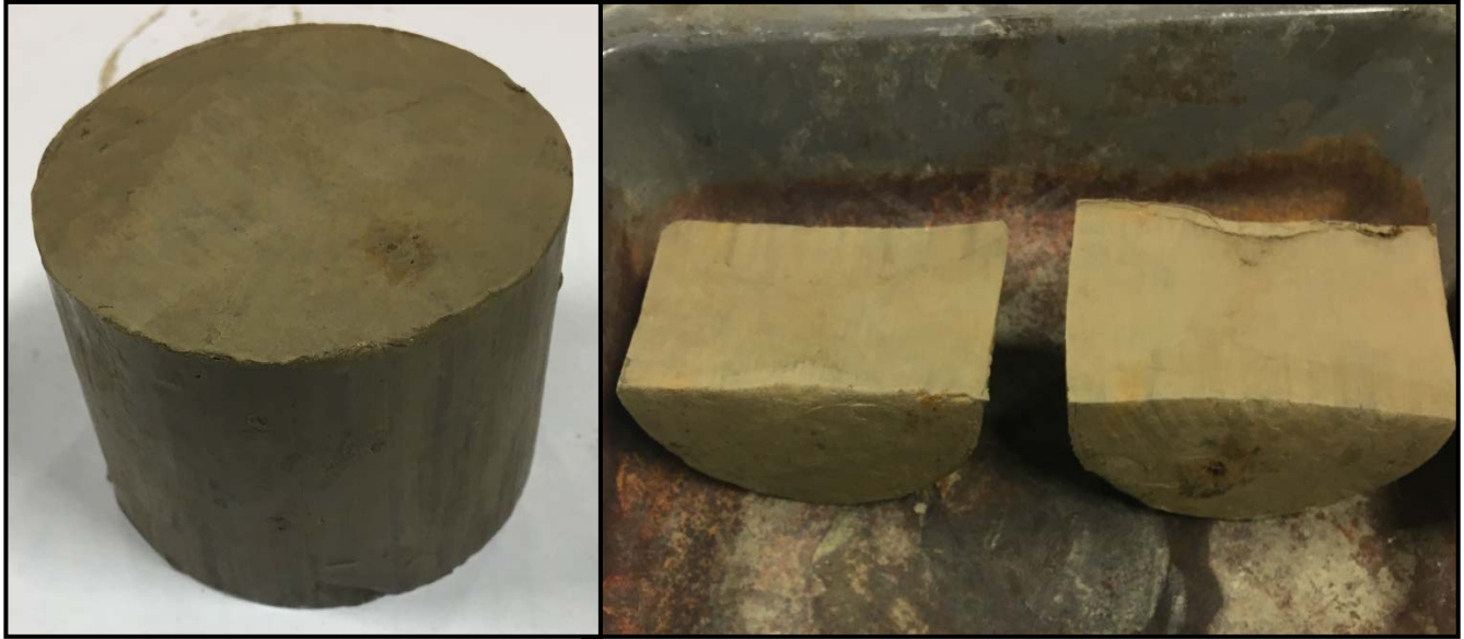
PHOTOGRAPH #3: Sample S3 after hydraulic conductivity testing.
