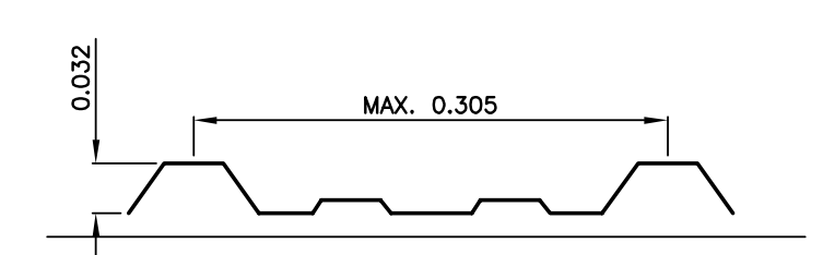
8 EXTERIOR LINER PANEL SCALE = 1:5
