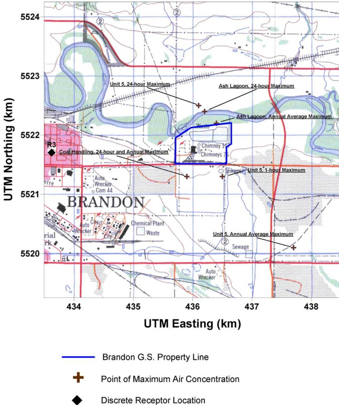
Figure 5-5 Maximum Predicted Incremental 1-hour Average NO<sub>2</sub> Concentrations (µg/m<sup>3</sup>) due to Unit 5 Emissions
