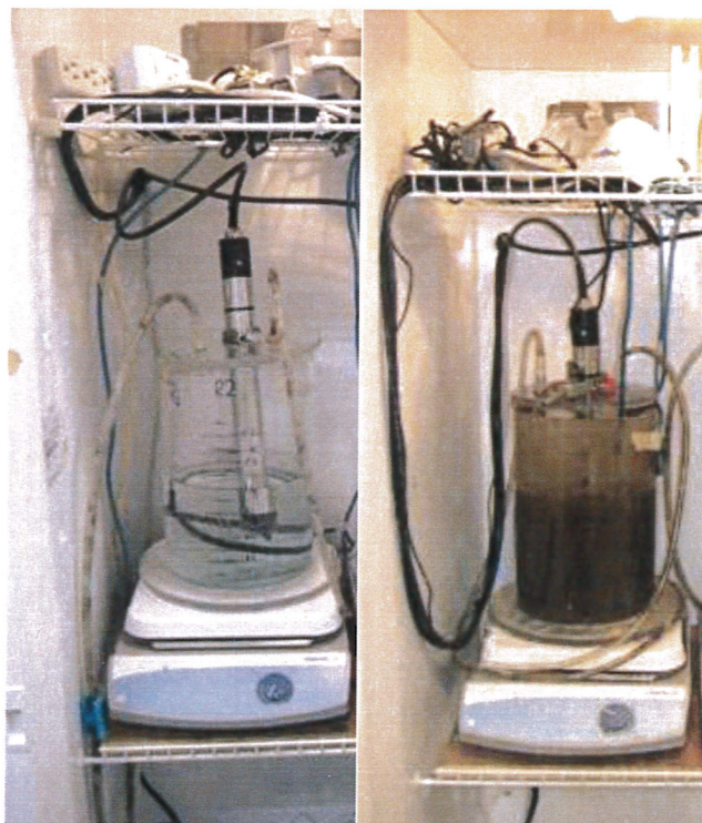
Figure 2.1 SBR Reactor before start on the left Reactor during program on the right
