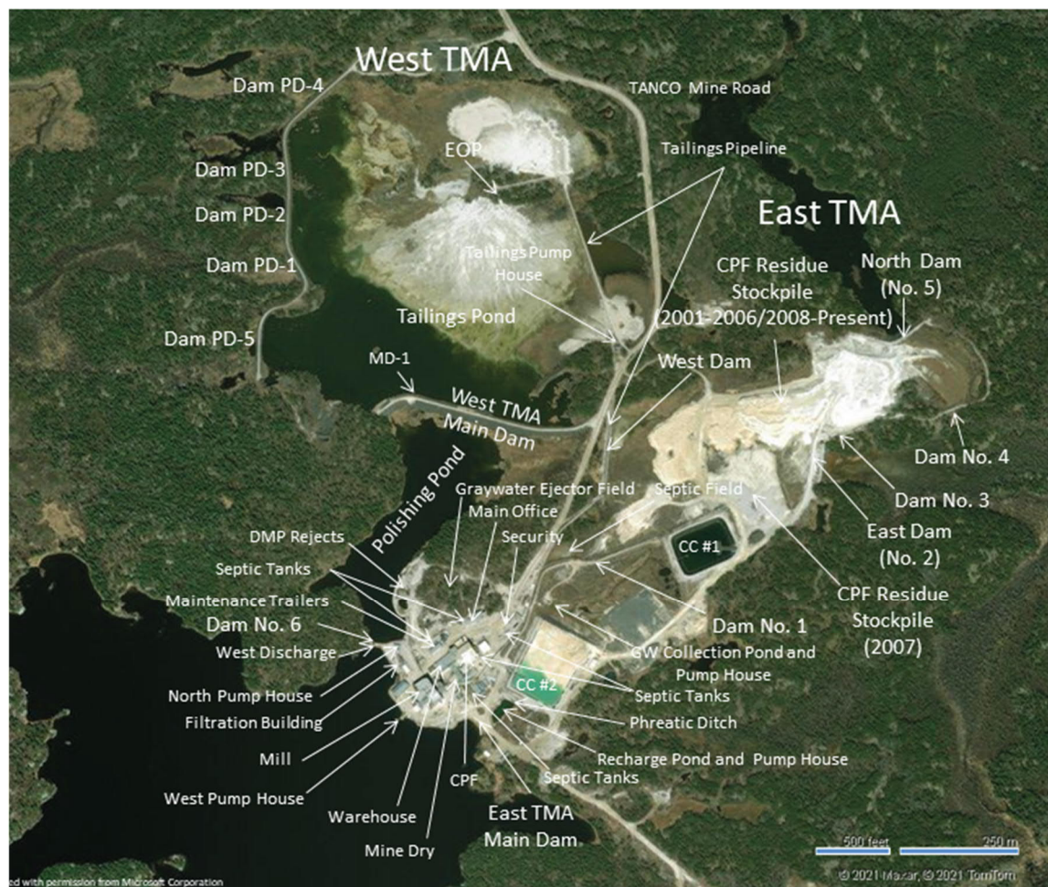
Figure 2-2: Existing TMA Infrastructure General Arrangement
