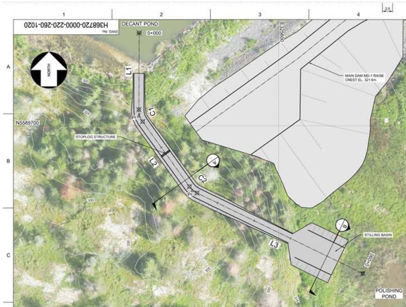
Figure 2-4 Tailings Pond spillway design (Hatch 2023a).
