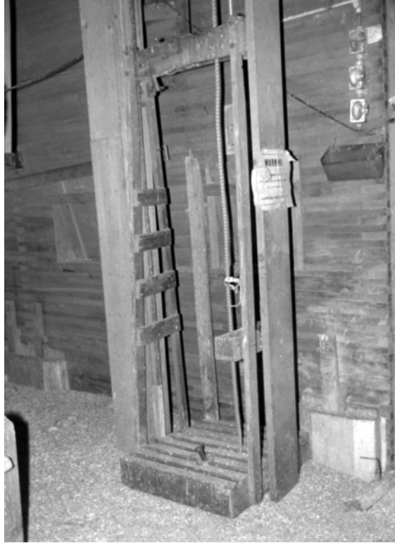
A rare example of an original wooden man-lift. The unit operated on a system of counter-balancing weights and provided the elevator agent with quick and easy access to the elevator head. Later examples, though similar in design, were constructed of steel. (Lenore 291.L.1)
