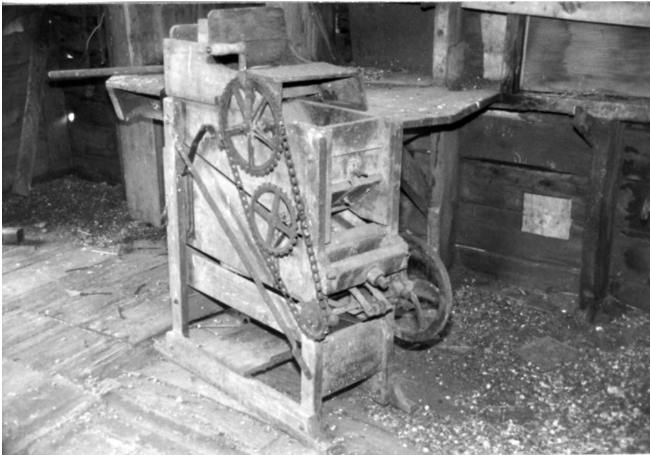
A rare surviving example of an early grain 'kicker'. This device was used to clean samples of grain being delivered to determine the amount of 'screenings' and other foreign material present. This in turn determined the dockage to subtract from the weight of the grain delivered. (Barnsley 726.L.2)
